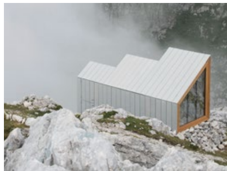
öko skin flex 147 mm, silvergrey, vertical installation, screwed on wooden substructure
